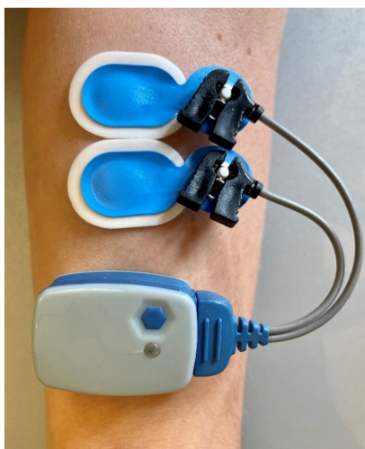
Figure 3: EMG electrodes and Noraxon EMG Sensor.
